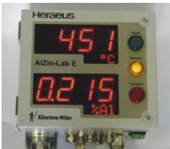
AlZin-Lab E may be connected to a dedicated PC or server PC via a serial Com port or via Ethernet (TCP/IP). Optionally Profibus and Modbus can be offered. The sent data strings may be used for in-plant logistics. The optional AlZinlog PC-software makes it comfortable to compute the measured data, and further process it in various Windows programs.
