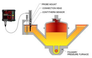
Contilab E for continuous measurements with a hot-zone cable connected to the temperature sensor.
