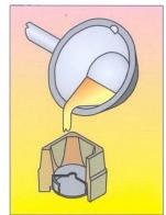
Cost of blast furnace slag sampling can be reduced considerably by using the blast furnace slag cup sampler. The blast furnace slag cup sampler provides a slag sample that can immediately be analysed in the lab. It avoids expensive slag sample preparation and saves a lot of time. The slag is collected by means of a special spoon. This spoon ensures that iron droplets sink to the bottom. The slag is cast into the cup. After a few minutes, the slag cup is crushed and the slag sample can be
