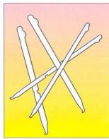
Evacuated Pin Tubes are used for sampling from spoon in ferrous and non-ferrous melts. They feature a thin wall bulb section which melts in contact with molten metal. The molten metal is sucked into the tube to form a solid slag free pin.
