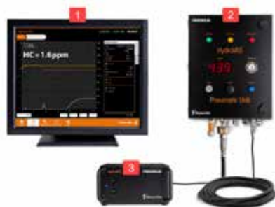
HydroVAS® system with (1) Screen, (2) Pneumatic Unit, (3) Processor Unit.
