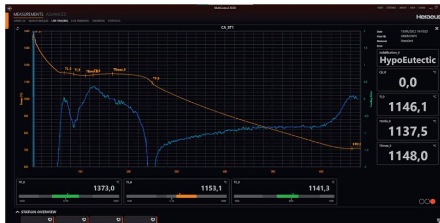
Live tracing view of measurement results
