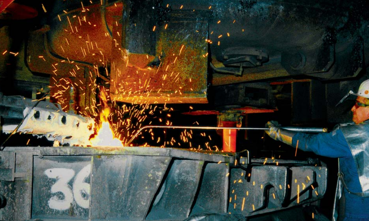
Bath temperature measurement in the tundish
